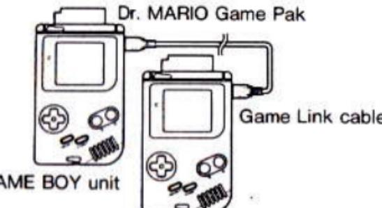
(1) Connect the Game Link cable as shown on the left and make sure that both Game Paks have been inserted correctly. Then turn both power switches ON at the same time.
